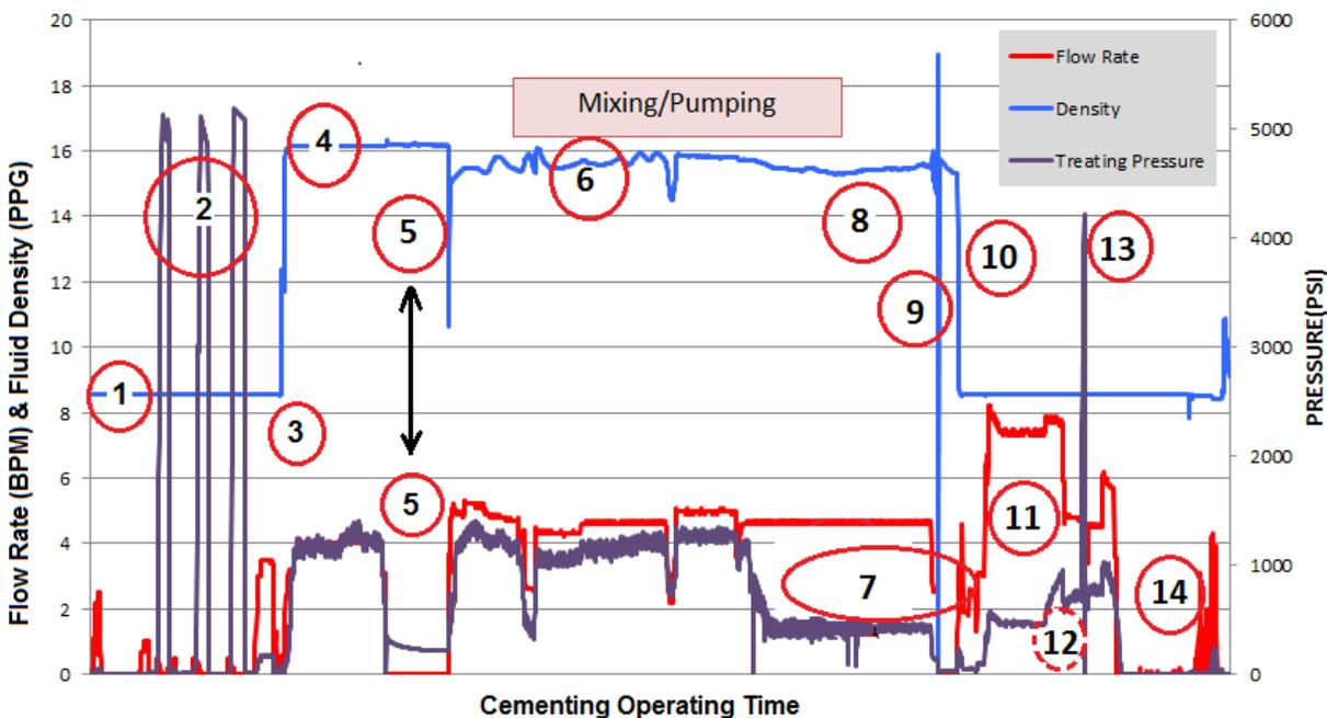
Figure 2 - Analysis of a cement job pump chart can show expected behavior or potential problem areas.
