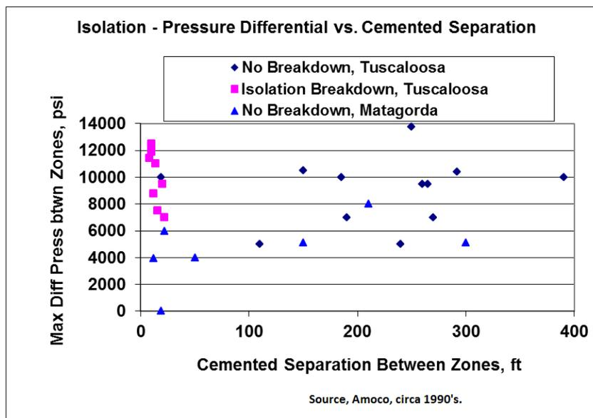
Figure 1 – Cement breakdown and isolation success for Tuscaloosa (on-shore) and Matagorda (Off-shore) gas fields.
