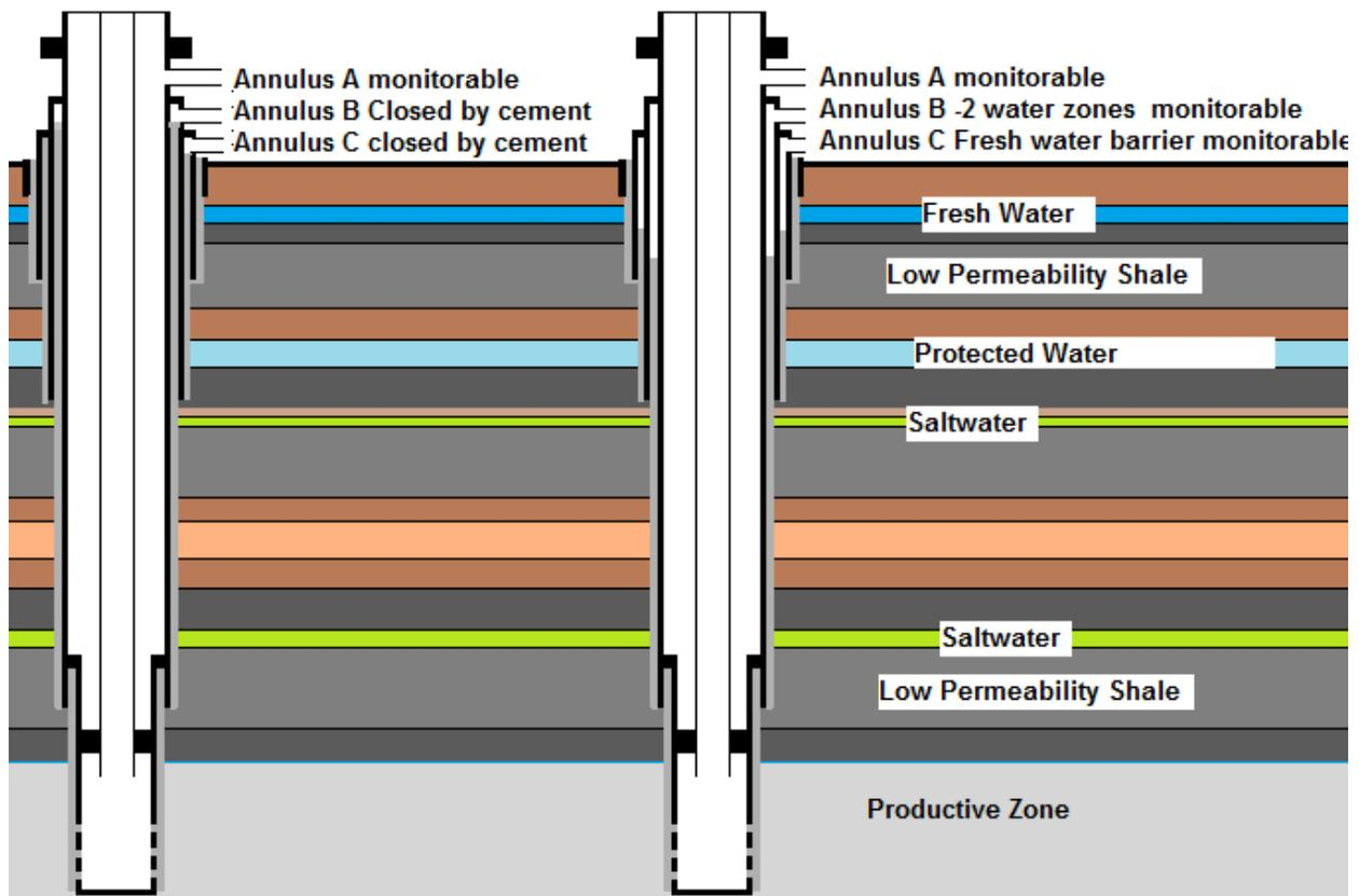
Figure 5 – Comparison of fully cemented and monitored annuli.
