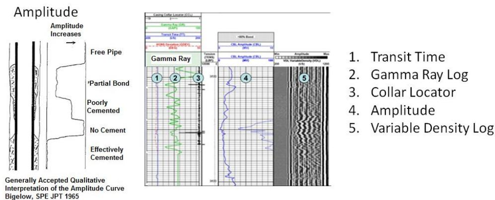
Figure 4 – the log tracks of a CBL.
