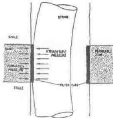
Basic concept of differential pressure sticking shows pipe is stuck in the filter cake of permeable zones.
