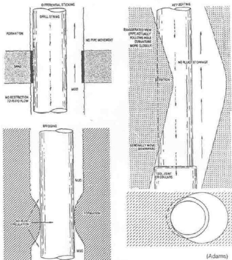
Figure 1.4: Top Left: Differential sticking-pipe held on wall by inward driving pressure. Pipe cannot move, but circulation is possible.
