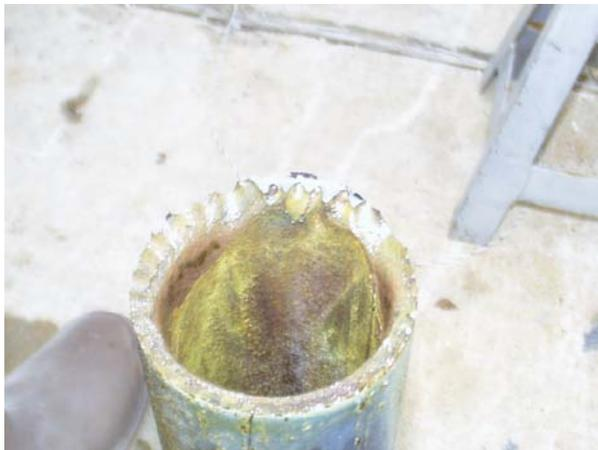
Typical applied tension to separate the pipe is usually between 20,000 and 50,000 lb. If effective tension cannot be applied (dogleg section or horizontal well), another type of cutter should be found.
