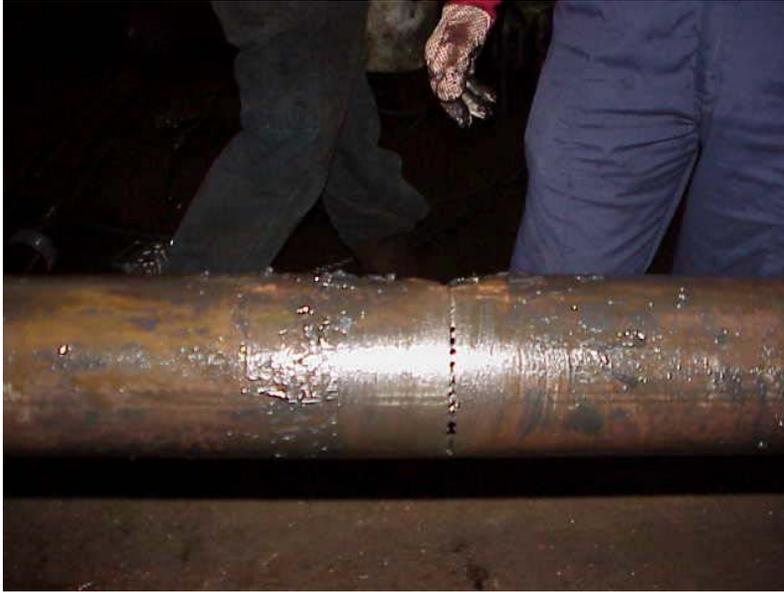
The tool body port size and condition influences tubing cut efficiency. Some chemical cutters are reused, thus the port size may be larger than optimum. Larger ports result in an inefficient spray pattern and a poor cut.
