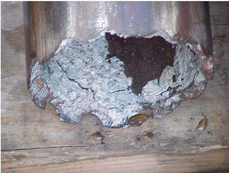
The impacted surfaces are melted. Incomplete cuts and misfires have been the major drawback, but some successes in chrome pipe have been recorded. The cutter has few limitations, however, outside casing strings may be damaged by application of the cutter.
