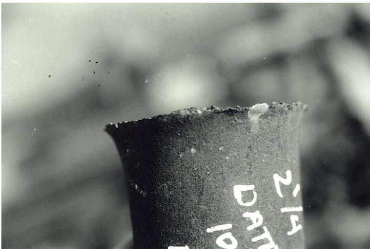
Early cutters produced large flares (20% pipe diameter growth or more) and broken sections of pipe. Later cutters (last few years) have been re-engineered to produce less than a 10% flare and no ribbons or splits.
