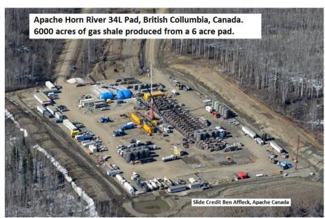
Twelve wells sit on 0.3 acre. Total developed footprint using horizontal multi-fractured wells is reduced by ~90% when compared to vertical well development of same area.
